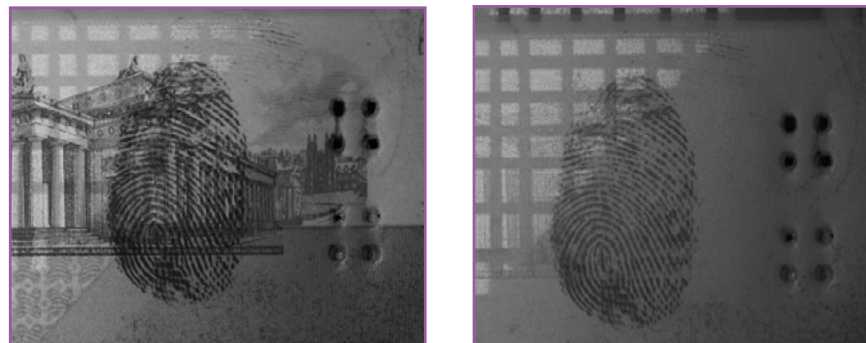
Figure 1. Fingerprint enhanced using black powder suspension, visualised under white light (left) and Infrared light (right).
